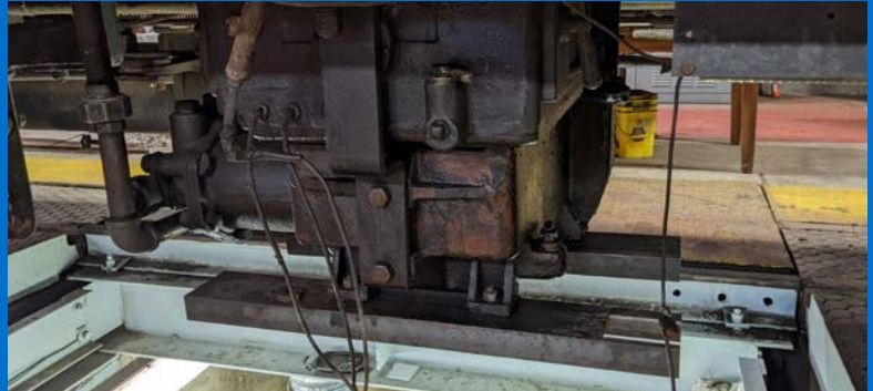
Railway car positioned with the air compressor over the pit in the shop
